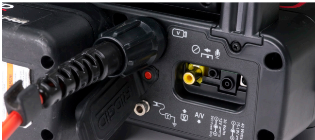
Figure 4 – Connecting the SeeSnake System Cable to the DVDPak2
