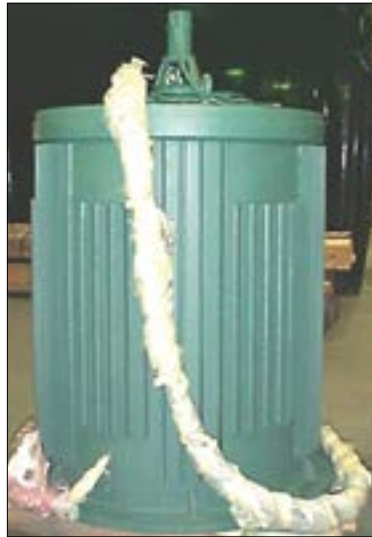
HP: 650 RPM: 900; Frame: V0840 Enclosure: TEAO; Application: Tunnel Ventilation Fan (to be located in the One World Trade Center - formerly known as the Freedom Tower) Industry: Air Handling
