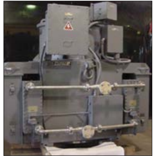
HP: 900 RPM: 1200 (with a 20 Hp, 300 RPM pony motor) Frame: V10840 Enclosure: TEWAC; Application: Moderator Pump Industry: Nuclear Generating Station
