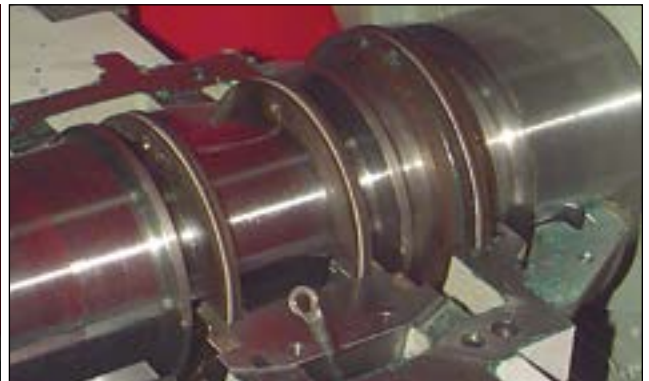
▲ Tilting Pad Bearing
