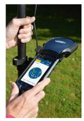
Insert the SP20 into the bracket so that it is pinched where you would normally hold it in your hand. That way you keep the rear camera clear and preserve access to the Power button.
