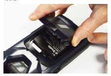
8. Then push the battery door against the unit and lock it.
