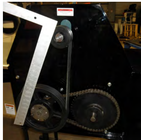
Lay a straightedge across pulley faces
