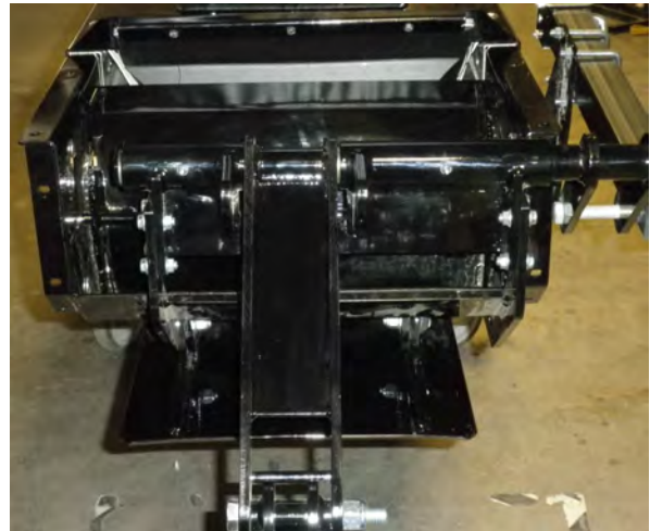
Bottom clean-out covers removed
