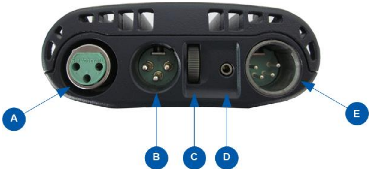
Figure 2-8: HBP-2X connectors and controls (rear view)
