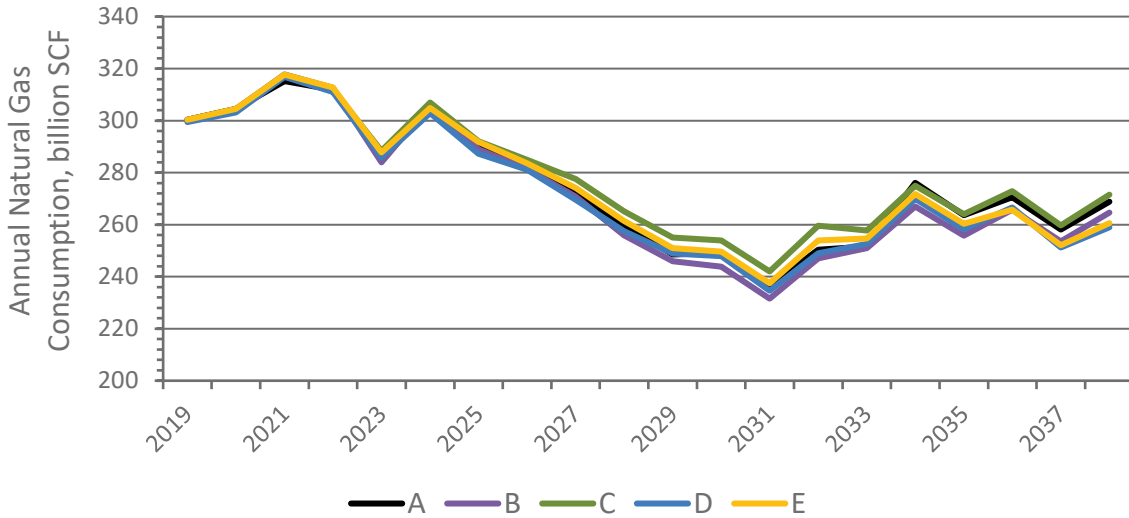
Figure 5-17: Trends in average annual natural gas consumption by alternative strategy based on averages of the six scenarios. The volume is based on the heat content of 1,033 Btu/cubic foot of natural gas used by the electric power sector in 2017 (USEIA 2018e).
