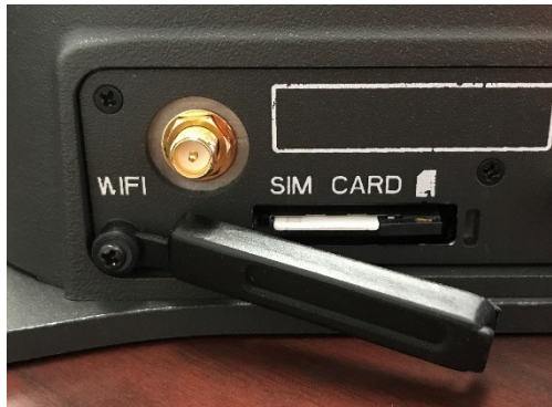
Figure 2-12 SIM Card with Cover Opened
