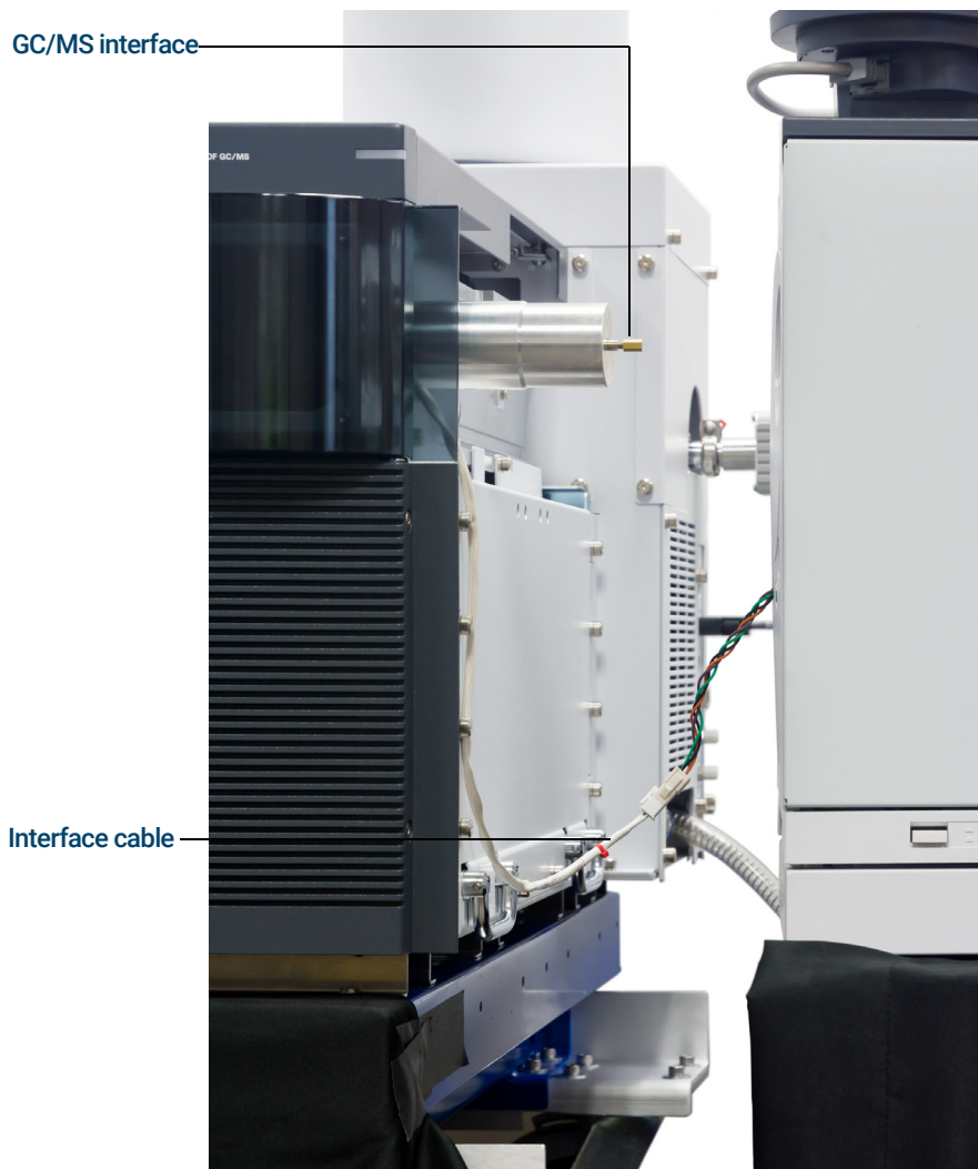
Figure 9. Separating/connecting the MS and GC
