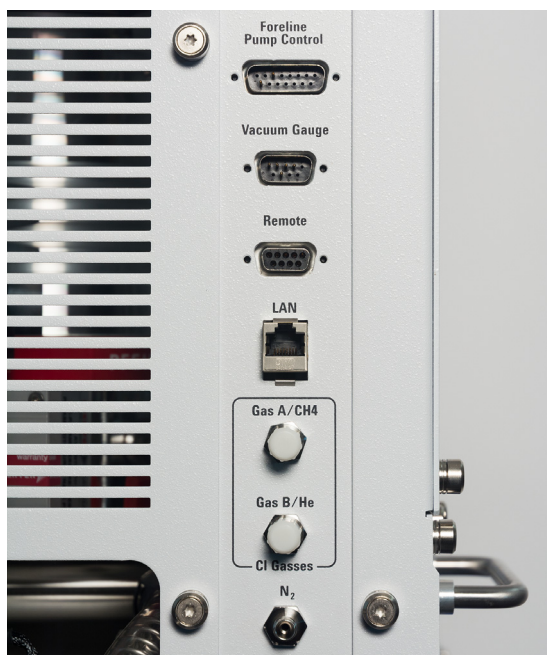
Figure 3. Back panel connections
