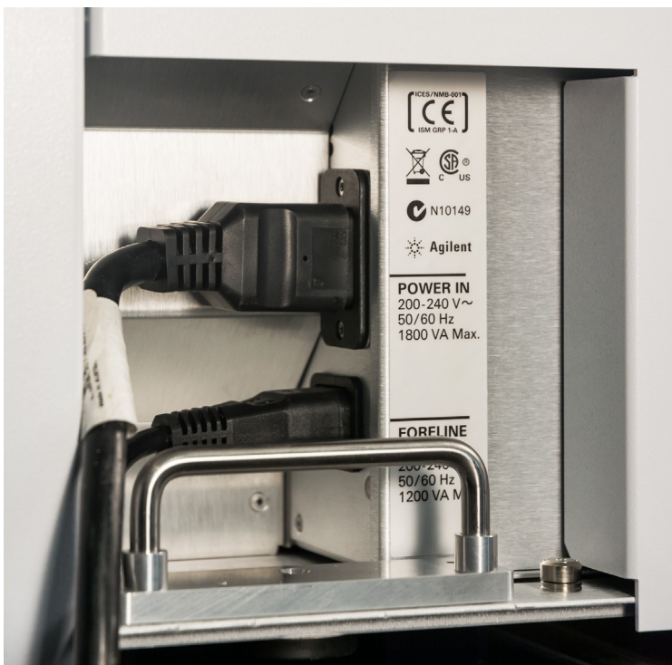
Figure 2. Side panel power supply
