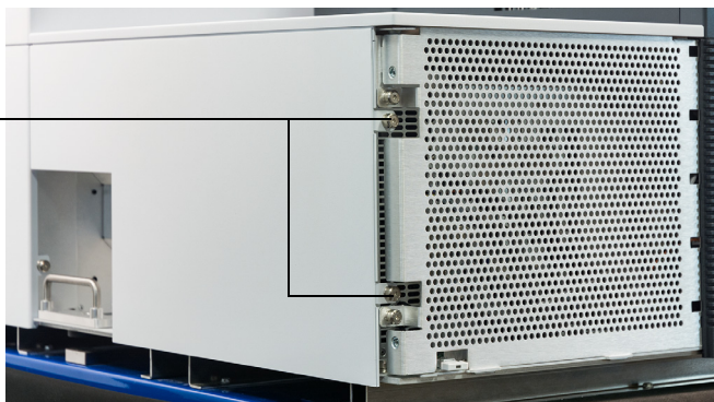
Figure 14. Left side cover captive screws
