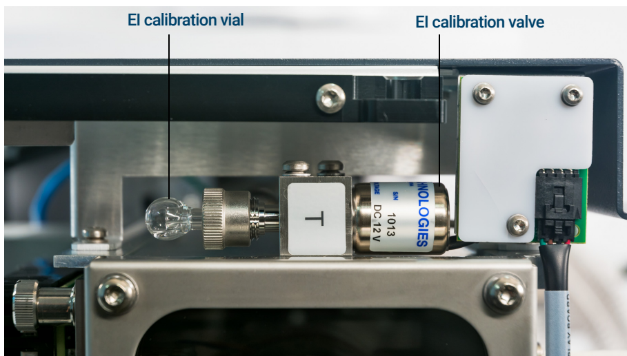
Figure 21. EI calibration valve
