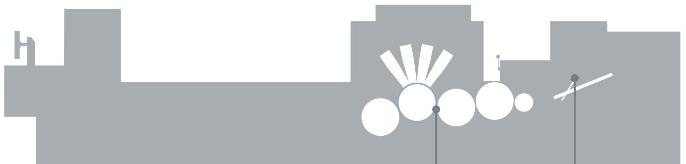
Real-time variable data processing – The Jet Press 750S has just 2.2 seconds to scan the front-side barcode and load data for the reverse side before the sheet reaches the printheads.
