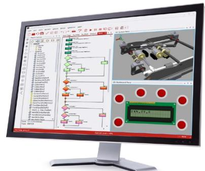
Simulation of car seat motor and actuator movement being controlled by MCU.
