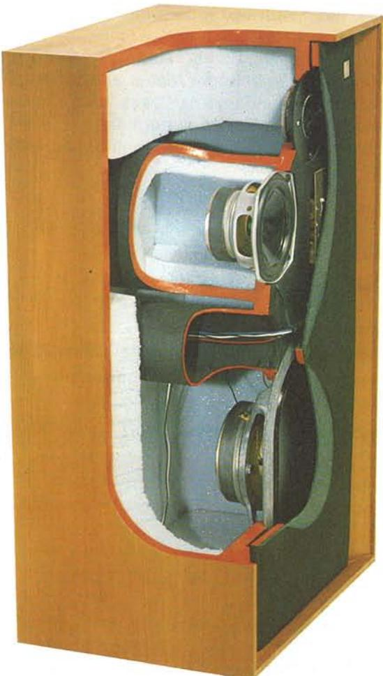
The Concerto is a vented speaker box of 62 litres, fitted with three drive units.
