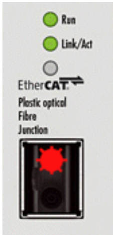
Figure: Transmitter channel in the EK1561 Be sure to observe the safety instructions [ ▶ 89 ] for class 1 lasers!
