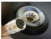
MIC shielded composite cable before connection to a MIC440 camera
