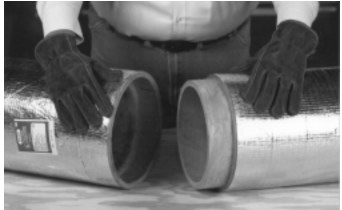
1. Preformed round duct sections are joined with male and female shiplaps. Joints are taped; staples are not required.
