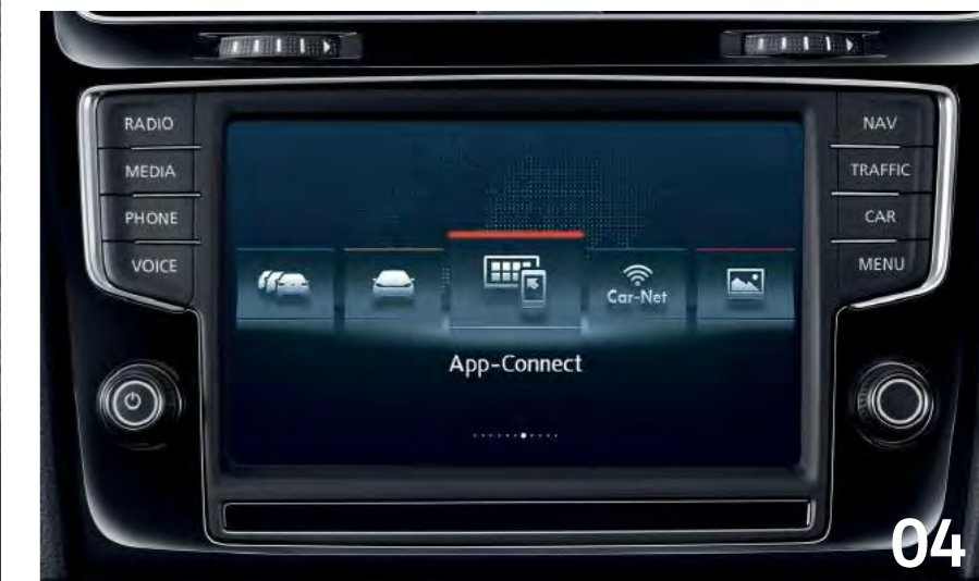
04 Car-Net 'App-Connect' 4 allows you to integrate a smartphone with your car by allowing 'mirroring' of the display on the infotainment touch-screen via USB connection. It uses the combined functionality of Apple 'CarPlay', Google 'Android Auto' and 'MirrorLink'™ to replicate the smartphone display, allowing operation of certified apps including audio and voice control (if supported by the app). Please note, there is usage of only certified apps while driving. Optional on all models. Car-Net 'App-Connect' is standard on Discover Navigation Pro touch-screen navigation/DVD radio system.
