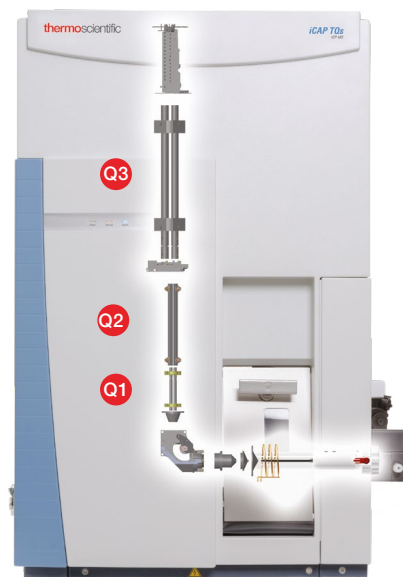
Figure 1. iCAP TQs ICP-MS. In TQ-O 2 triple quadrupole mode, Q2 (collision/reaction cell) is pressurized with oxygen as a reaction gas, Q1 is set to the analyte mass (M + ) and Q3 is set to the product ion mass (MO + ) or (M + ).
