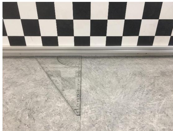
Finding a line perpendicular to the wall
