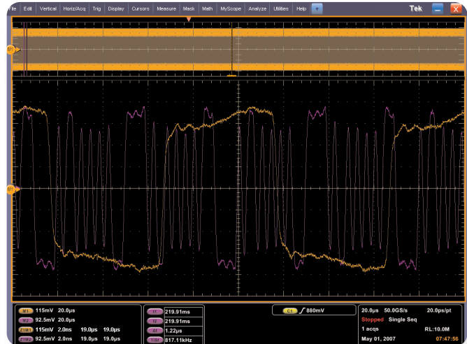
▶ Figure 14. Acquisition of RefClk and Data using Dual Port method.
