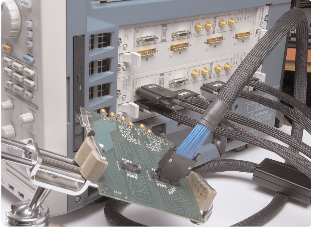
▶ Figure 31. The mid-bus serial probe connects to dedicated test pads on the circuit board's surface, consuming minimal board real estate.
