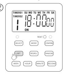
Short press the SET button, then press WEEK, HOUR, MINUTE, SECOND to set the required boot time of the first group. (Note: When setting, you could press CLE/RETU to clear the current data and set again. If your data is cleared by mistake, please press CLE/RETU to restore)
