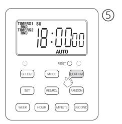
After setting, press CONFIRM button, the device will start to work according to the set time of the timer. If you do not press CONFIRM, you can continue to set the timer for the second group and the third group, or even more groups.
