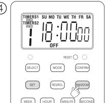
During setup, you can press the RANDOM button to select whether you use the RND holiday mode. (Note: The RND mode can only be selected when the timing is set. After pressing the CONFIRM button and it starts to work, you can't select RND again. You need to go back to the timing setting state to select RND)
