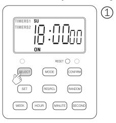
Short press the SELECT button to select TIMER1, TIMER2 or TIMER1&TIMER2, and make it or them to work. (Note: TIMER1 indicates the socket on the left side and TIMER2 indicates the socket on the right side)
