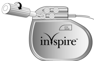
Figure 16. Tighten the two lower setscrews
