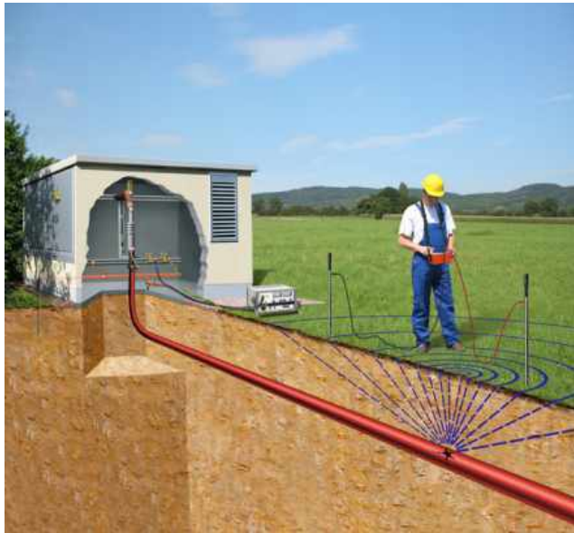
Fig. 12: Principle of the pinpointing with voltage gradients
