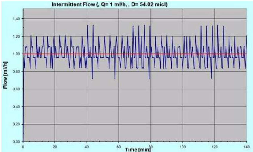
Figure 12.2. Trumpet Graph, Second Hour of Delivery, 1 mL/h
