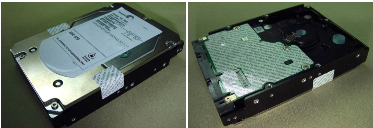
Figure 11. Example of FIPS tamper evidence labels.
