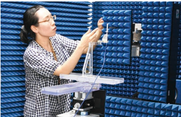
Example of OTA testing technology: Near-field test with a massive MIMO antenna
