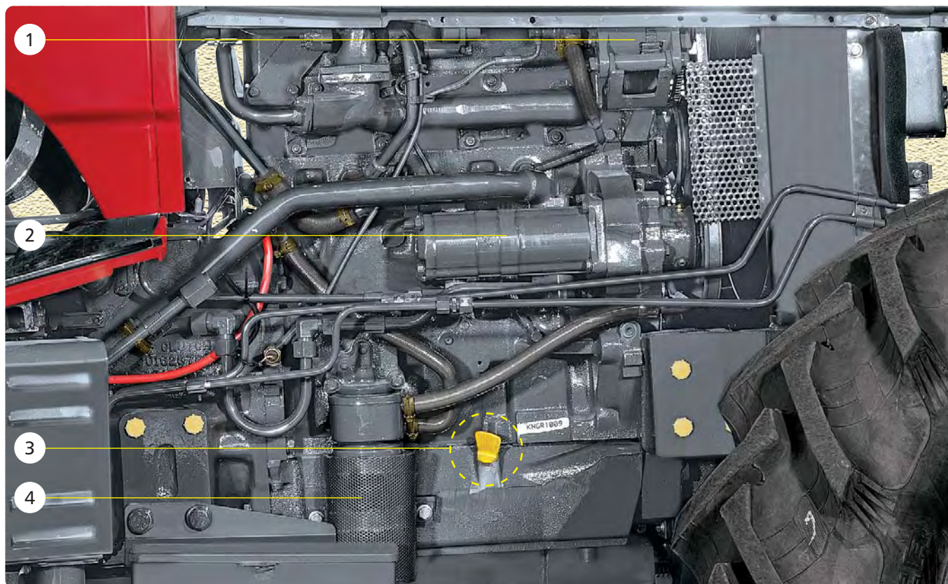
RH View : 1. Alternator 2. Hydraulic Tandem Pump 3. Dipstick 4. Oil Filter Engine
