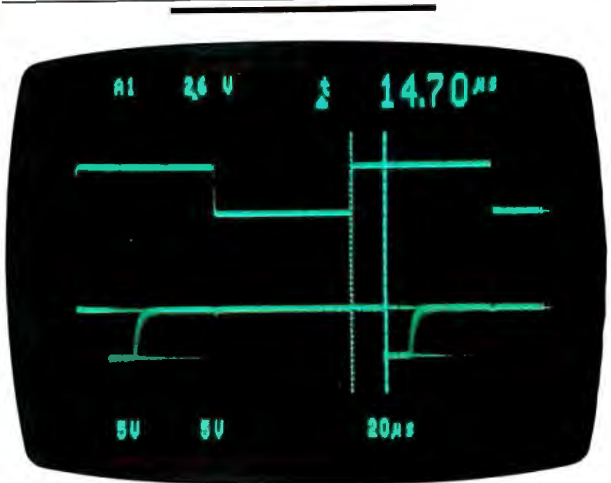
Photo 5: An oscilloscope shot of a simple interrupt response on the Model 50.
