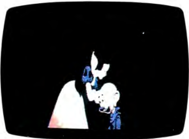
Photo 6: A reverse mask to photo 4. Now you can colorize pixels mapped to palette positions greater than 15.
