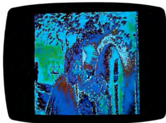
Photo 2: A straightforward mapping of gray scale to EGA color-palette values. Each pixel in photo 1a is divided by four, and the integer result picks that pixel's color-palette value.
