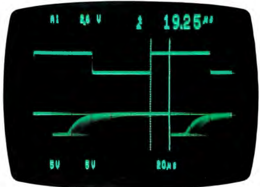
Photo 6: An oscilloscope shot of a simple interrupt response on the PC AT.
