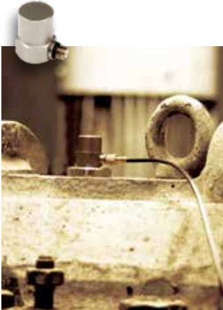
Type 4393 – robust charge accelerometer for high-temperature, light-structure tests
