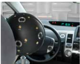
Spherical beamformer used for in-vehicle measurements
