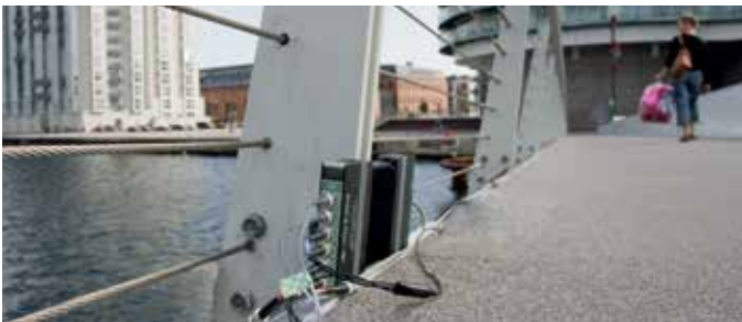
Distributed LAN-XI modules facilitate operational modal analysis of large civil engineering and mechanical structures
