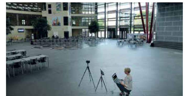
Room acoustics measurements using Type 2250, DIRAC Room Acoustics Software and the stand alone Echo Speech Sound Source
