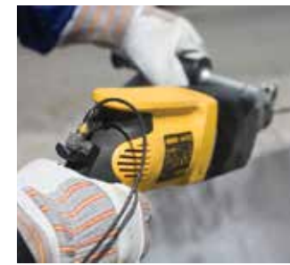
Triaxial hand-arm vibration measurement
