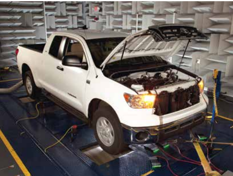
Our flagship test centre near Detroit is a state-of-the-art facility that includes a hemi-anechoic, four-roll chassis dynamometer
