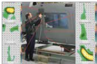
Hand-held array with position detection system using SONAH
