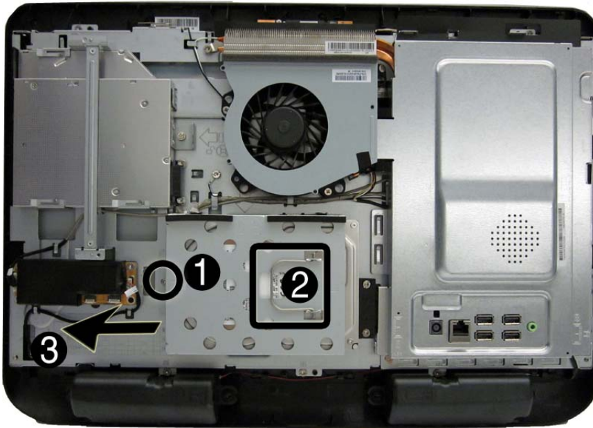
Figure 7-15 Removing the hard drive cage assembly
