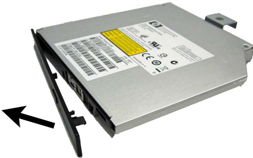
Figure 7-13 Removing the optical drive bracket
