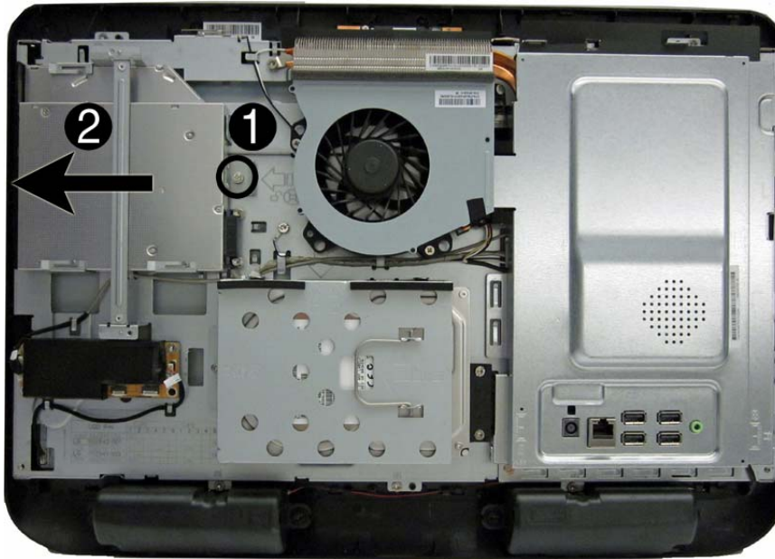
Figure 7-11 Removing the optical drive
