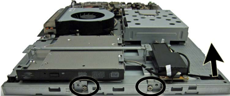
Figure 7-40 Removing the display panel screws and converter cable
