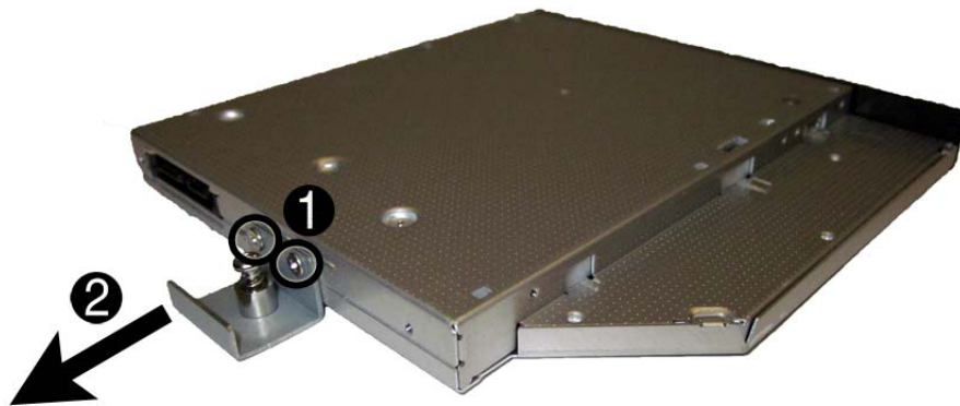
Figure 7-12 Removing the optical drive bracket
