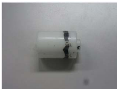
Soiling which can be peeled off by scratching with finger nail
