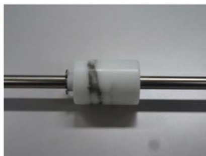
Soiling which cannot be peeled off by scratching with finger nail
