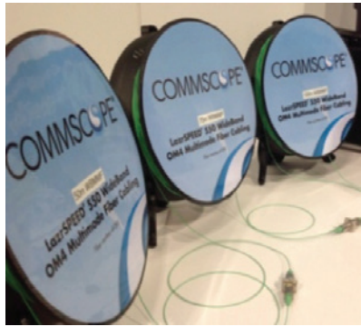
Figure 9 - 4 x 25 Gb/s WDM over 225 m of LazrSPEED 550 WideBand MMF at OFC 2015
