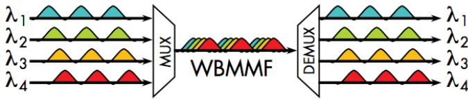
Figure 5 - WDM concept showing four wavelengths
