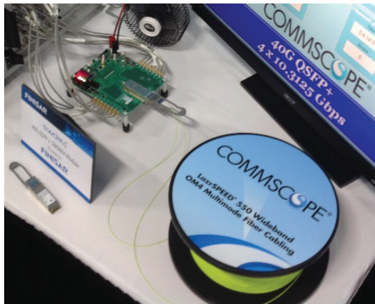
Figure 10 - 40G-SWDM4 over 500 m of LazrSPEED 550 WideBand MMF at BICSI
