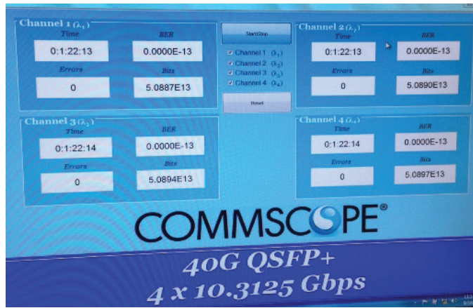
Figure 10 - 40G-SWDM4 over 500 m of LazrSPEED 550 WideBand MMF at BICSI
