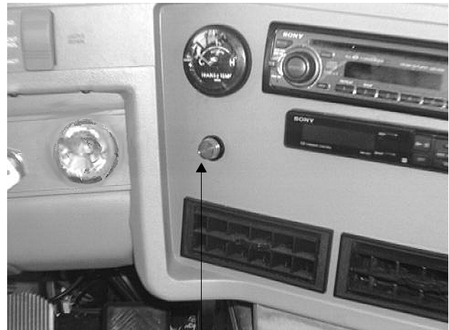
“Check Antenna” Light
