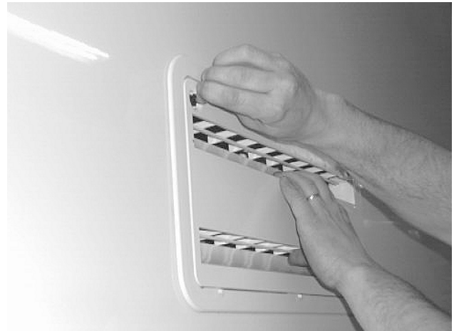
Turn latches open with coin
