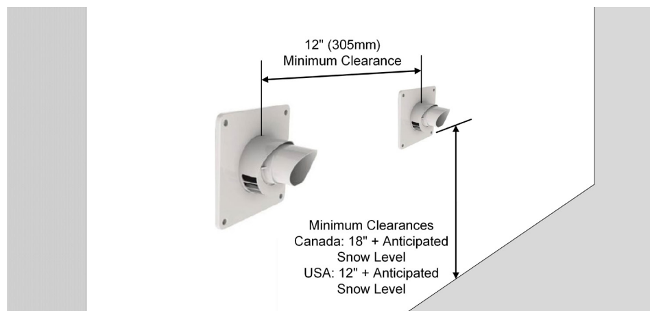
Figure 11a: Horizontal Concentric Termination - Two Kits
