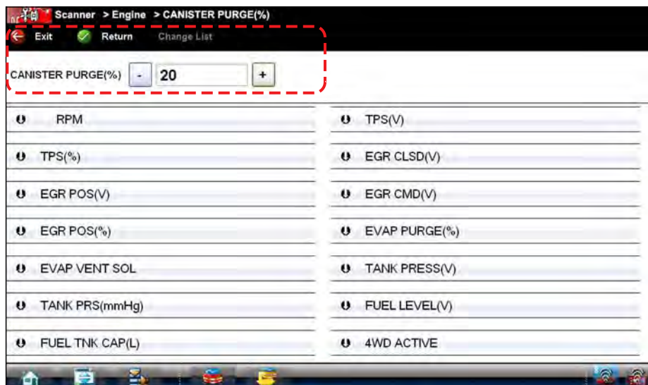
Figure 5-21 Sample functional test controls
