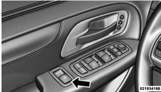
Power Vent Window Switch Open/Close
