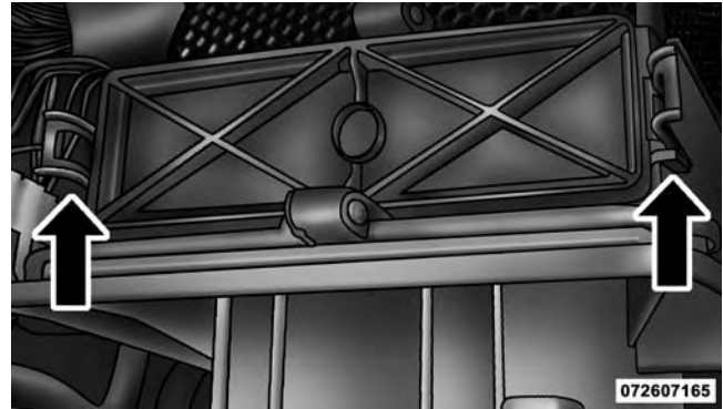
A/C Air Filter Replacement
