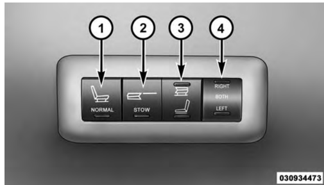
Rear Panel Power Switch Bank
