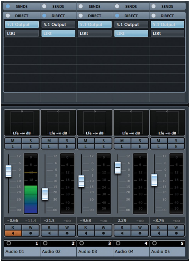
Figure 6.81 Direct Routing rack
