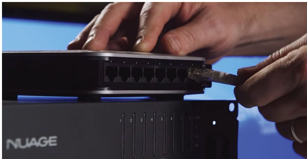
Figure 2.5 Connecting the Nuage system to a Gigabit Switch
