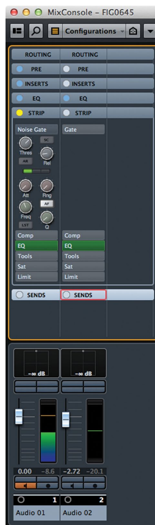
Figure 6.72 Strip Rack with activated gate
