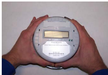
Figure 7 – Removal of Electronics Housing
