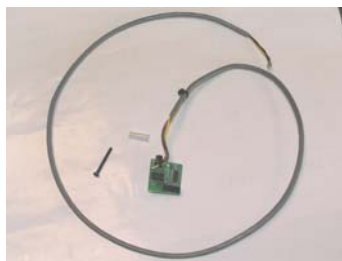
Figure 19 - KYZ Board/Cable, Mounting Screw and Spacer
