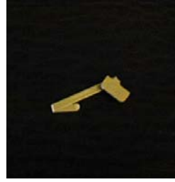
Figure 10 – Formed T- Seal After Installation
