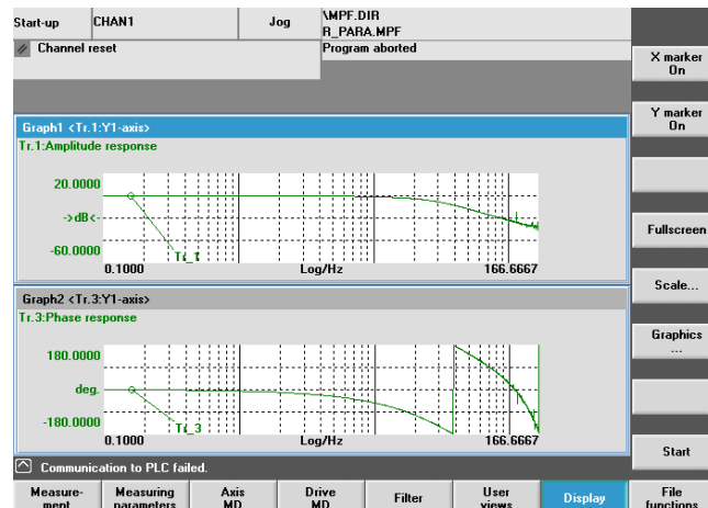
Figure 8-24 Optimized position control loop
