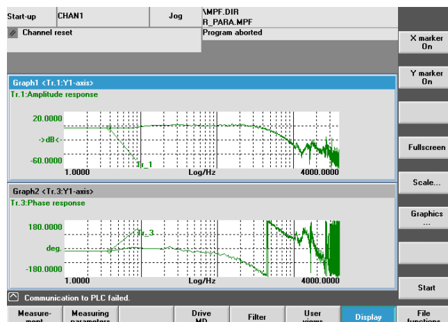
Figure 8-23 Optimized speed control loop
