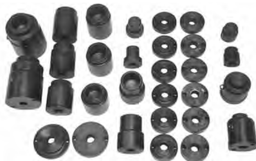
Contact tools and saddles required to service nine machine models in nine-inch pitch track group
