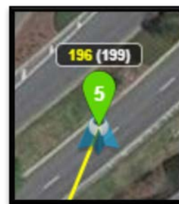
Figure 31 - Above Ground Waypoint Altitude
