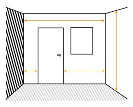
**01** Start by measuring from the floor to the ceiling. Then measure the distance between walls and from the corners to the doors.
