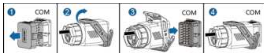
Figure 5-26 Securing the signal cable connector
