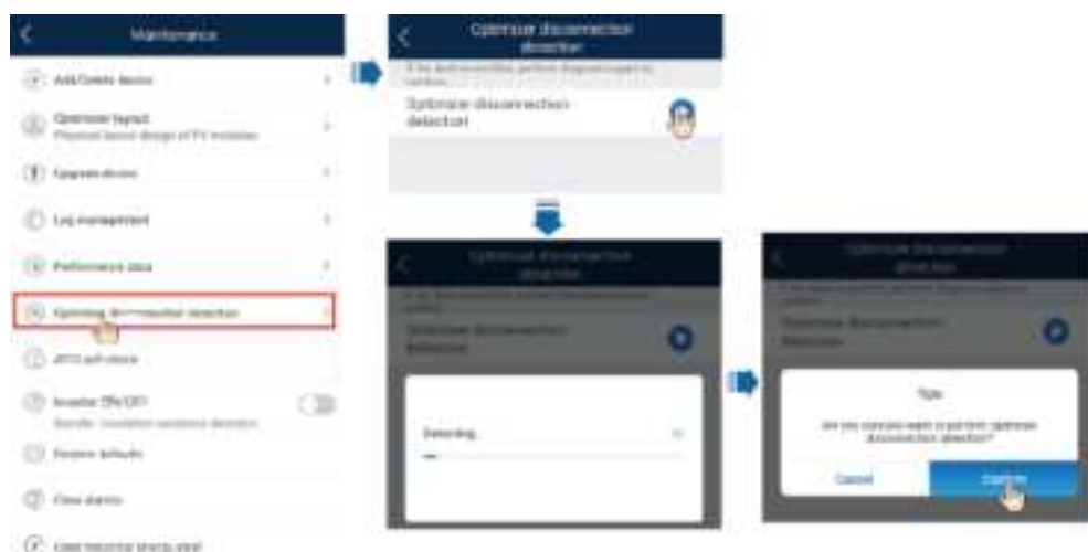
Figure 7-9 Detect optimizer disconnection
