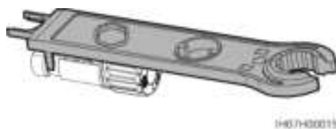
Figure 5-14 Removing DC connectors
