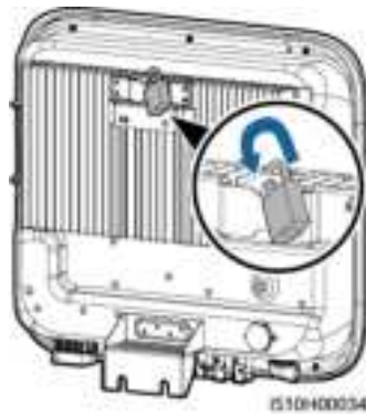
Figure 4-18 Installing an anti-theft lock
