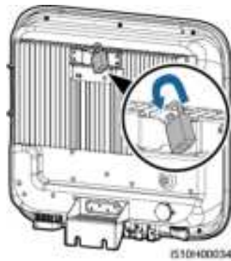
Figure 4-12 Installing an anti-theft lock
