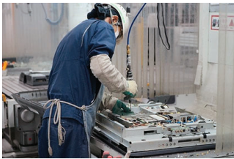
TV being dismantled at Green Cycle Corporation
