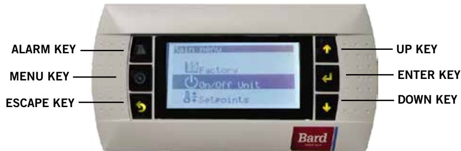
FIGURE 2.6 Bard-Link™ Controller Display
