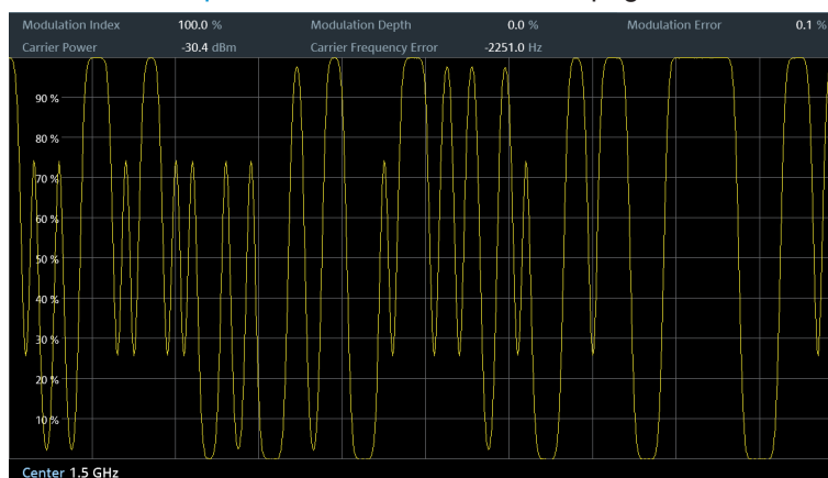
Figure 12-4: Modulation depth of a 2ASK signal
