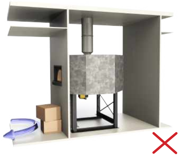
Blocked Air Vent
