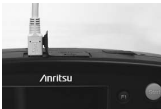
Figure 1.5.5-4 USB (Type B) Port
