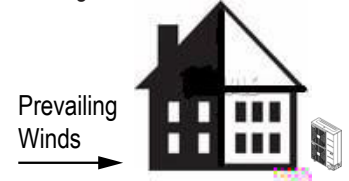
Figure 54: Leeward Side of the Building.
