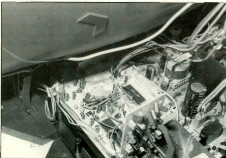
Figure 4. If the problem appears to originate in the video section, locate the large video processor or IC and observe critical waveforms.
