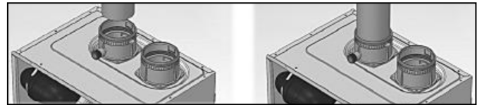
Figure 19 - Correct Installation into the Appliance Collar
