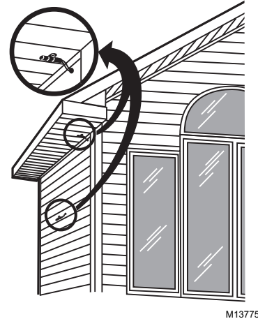
Fig. 7. Outdoor temperature sensor installation.
